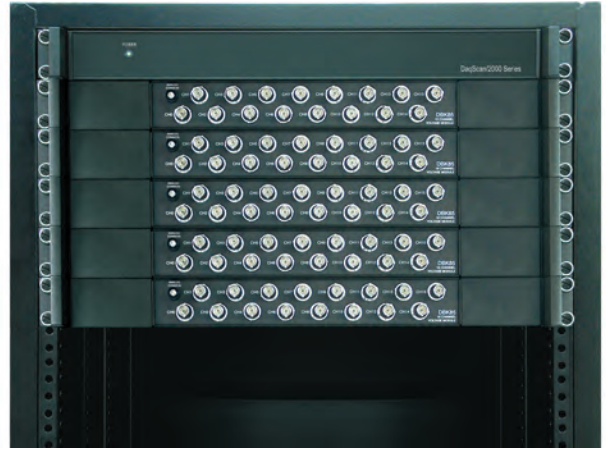
The 80-channel high-speed scanning system consists of an OMB-DAQSCAN-2005 plus five OMB-DBK85 16-channel voltage scanning modules. All channels can be measured at the maximum rate of 5 \mu s/channel
