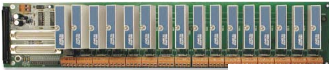
OMB-CA-37-1 (2) OMB-DBK207 and/or OMB-DBK207/CJC (3) signal conditioning and expansion board for 5B-compatible analog I/O modules; analog input expansion; mounted using Rack3
