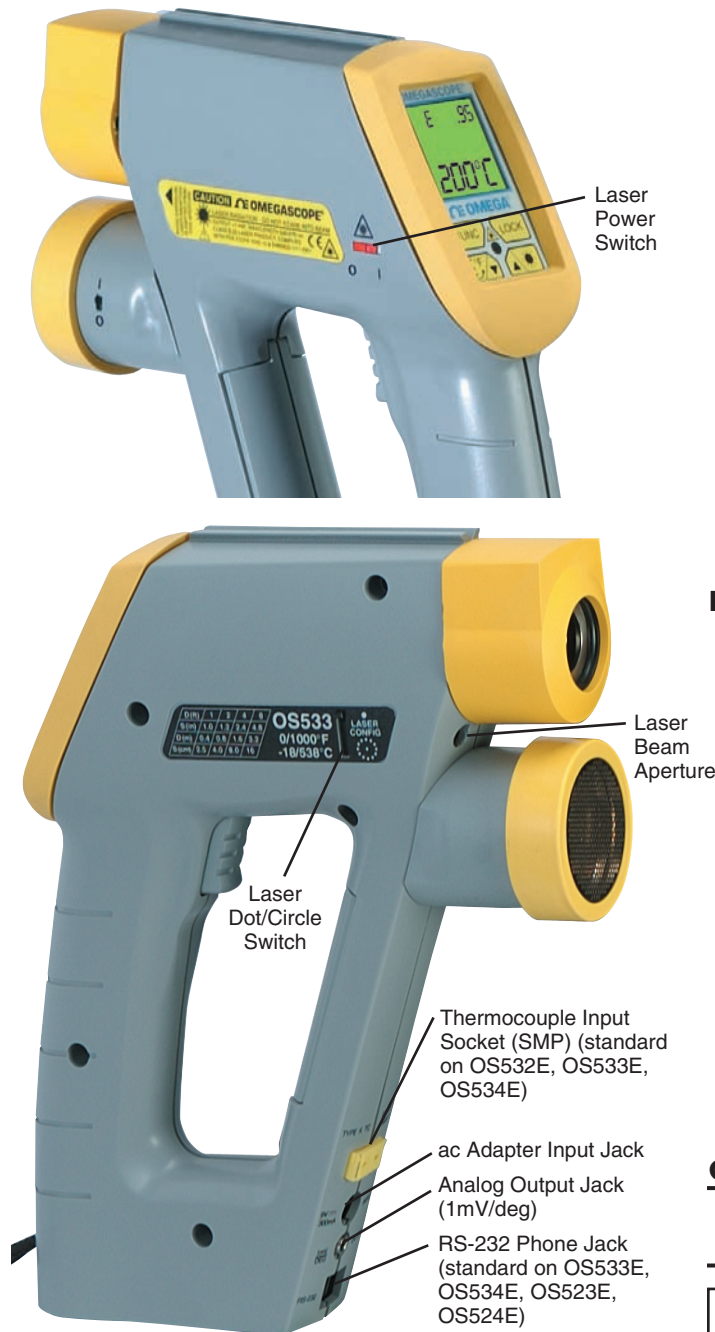
Figure 2. OS530E/OS520E Series Handheld Infrared Thermometer Various Views
