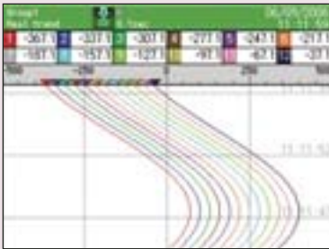
Real Time Trend Screen Display data (measured and virtual) of selected group. Vertical trend and horizontal trend.
