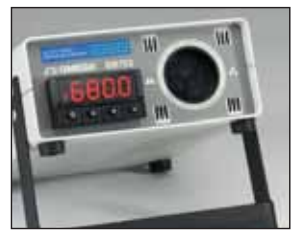
Model BB703 90 to 752°F, 1.125" Target Plate 0.95 Emissivity
