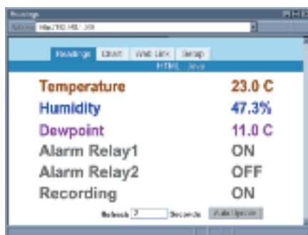
Readings through embedded Web server
