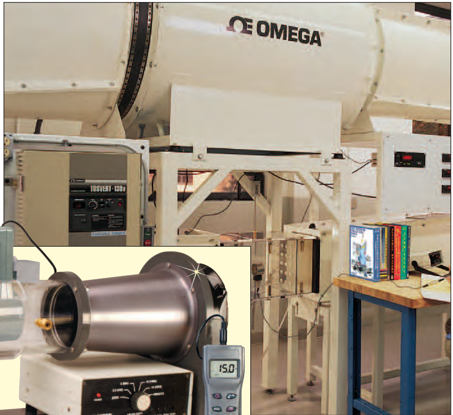
OMEGA's laboratory-grade large temperature-controlled recirculating wind tunnel.
