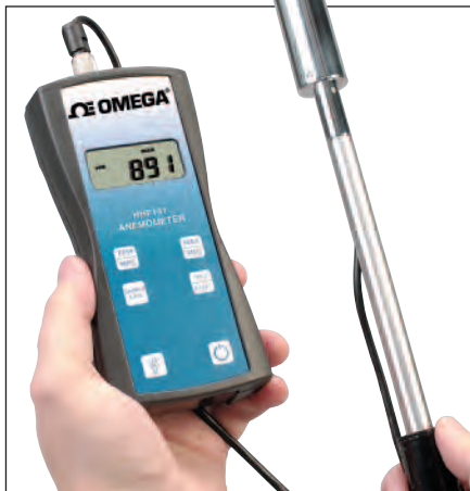
HHF141A microprocessor-based handheld air velocity meter, comes complete with 25 mm (1") dia. vane probe, flexible, straight and handle extension rods, 1.5 m (5') cable, 3 "AA" alkaline batteries, hard carrying case and operator's manual, $795. Visit omega.com/hhf141 for details.
