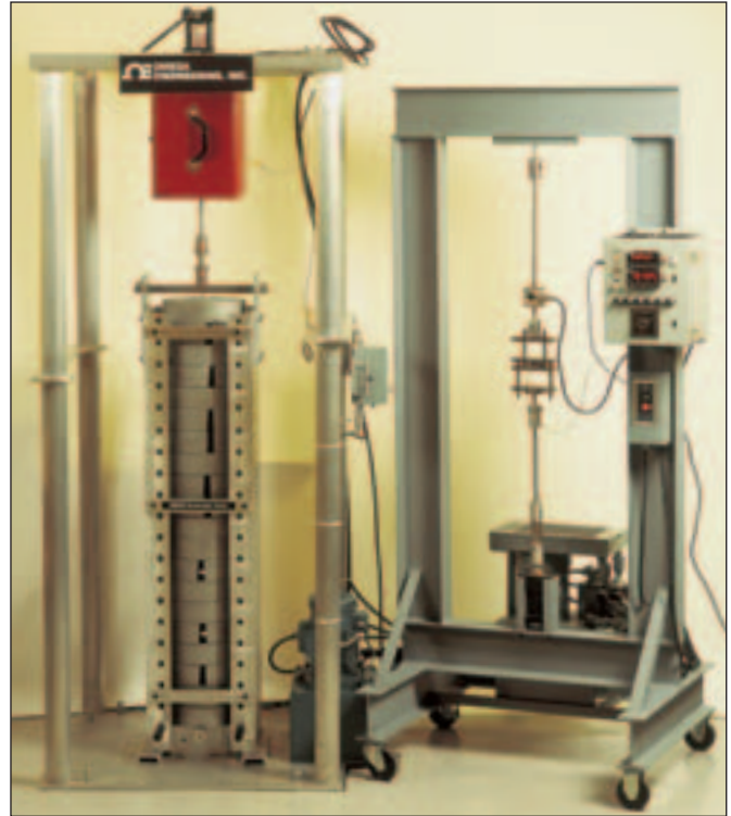
OMEGADYNE®, located in Columbus, Ohio maintains in-house state-of-the-art NIST traceable calibration standards for all your load cell and strain gage calibration needs. Pictured above is a high capacity dead weight tester (left) and hydraulic tester (right).
