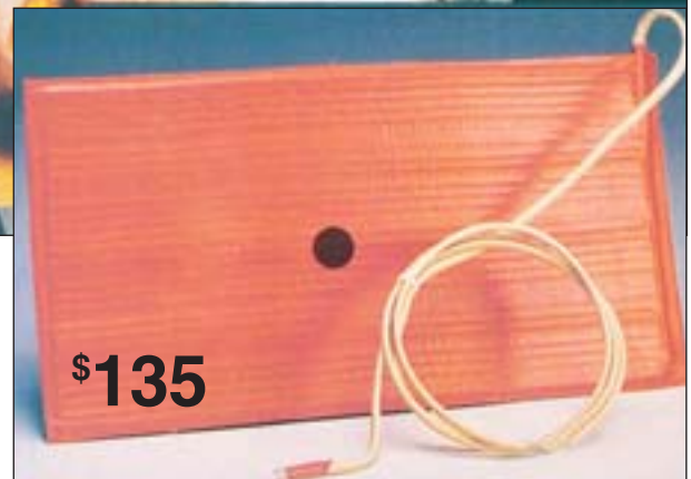
A Standard SSHB Series Silicone Rubber Heating Blanket Is Modified to a 305 x 406 mm (12 x 16") Size with a 25 mm (1") Diameter Access Hole in the Center for This Electronics Test Application
