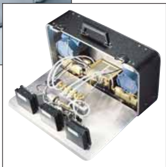
Pressure Transducers and Panel Meters Mounted in Carrying Case Permit Easy Calibration Checks at Remote Locations
