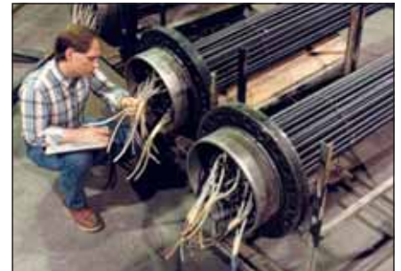
300 kW Flanged Immersion Heater Custom Designed for Heating Gases up to 538°C (1000°F) $14,595
