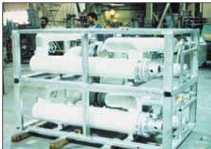
Two Custom Engineered Skid-Mounted Circulation Heaters, for Heating Lubricating Oil $26,375
