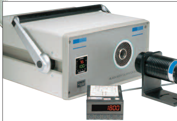
Shown calibrating the OS1552-A pyrometer, $690. See page J-71 for details.
