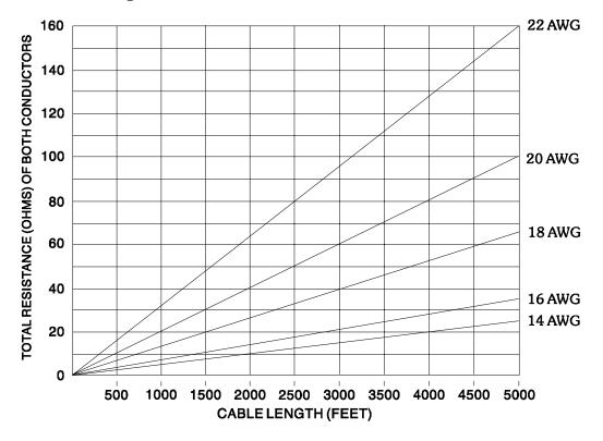
Figure 2-8 - Cable Lead Length Vs. Total Lead Resistance
