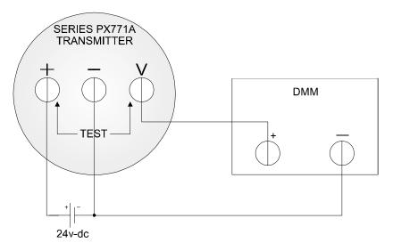
Figure 3-1a - Calibration Test Setup (Voltage Configuration)
