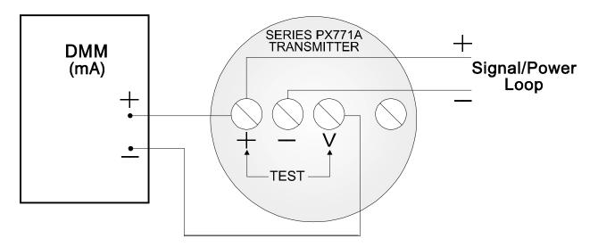
Figure 4-1 - Using Internal TEST Terminals to Measure Current
