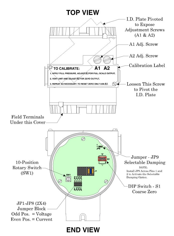
Figure 3-2 - Calibration Adjustments
