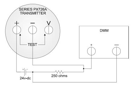
Figure 3-1b - Calibration Test Setup (Current Configuration)
