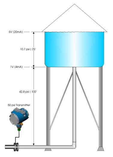
Figure 3-3 - Water Tower Level Measurement - Zero Suppression
