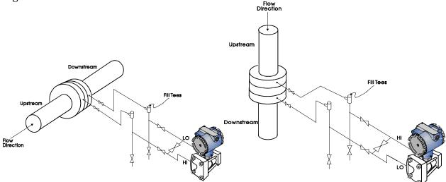
Figure 1A-11 - Steam Process, Horiz. Pipe Figure 1A-12 - Steam Process, Vert. Pipe
