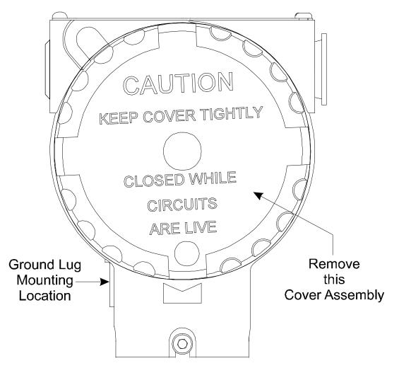
Figure 2-1 - Transmitter Cover Assembly Removal
