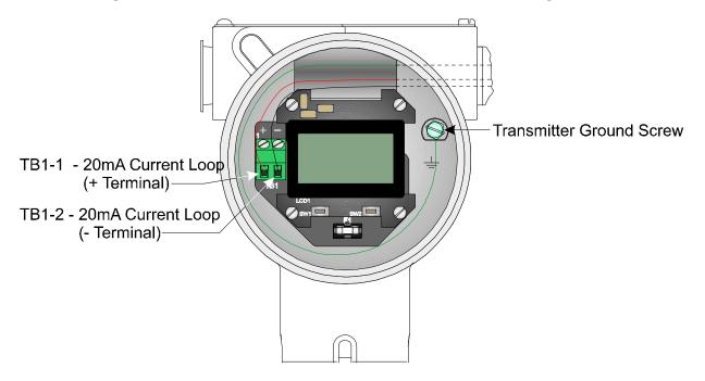
Figure 2-5 - Transmitter LPI Option Field Wiring
