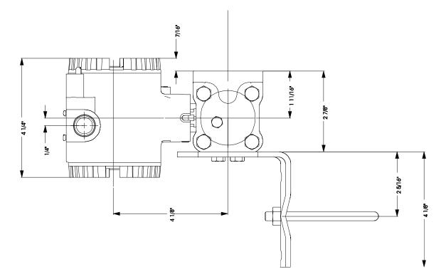
Figure 1A-4A - Overall Dimensions for Series PX771A Transmitter (With Flange Type Mounting Bracket
