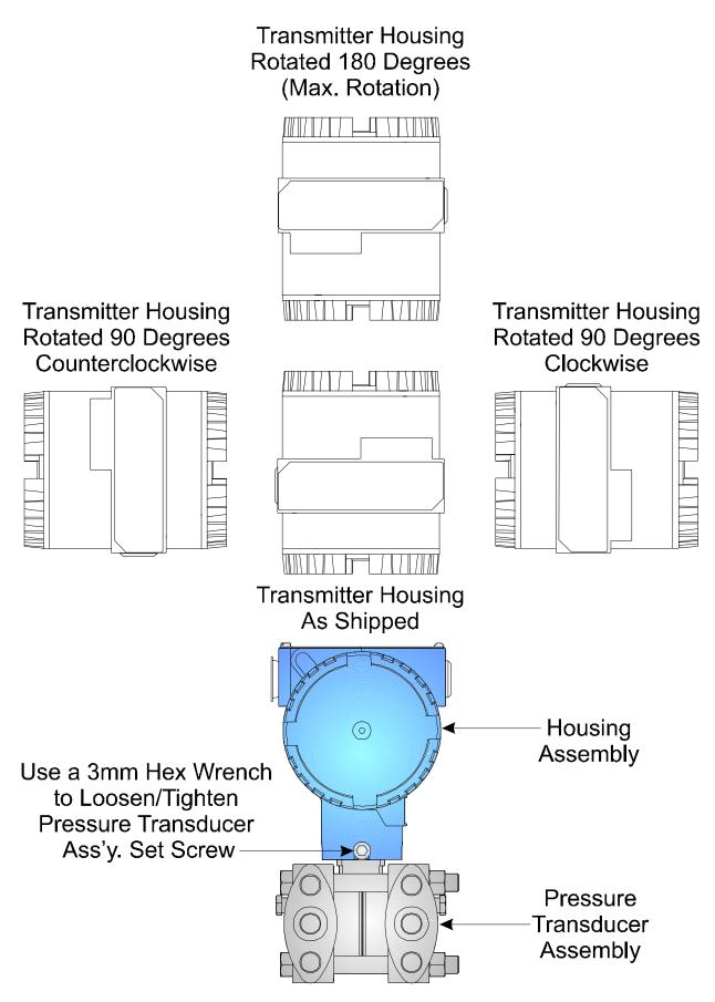
Figure 1A-6 - Transmitter Housing Rotation Diagram
