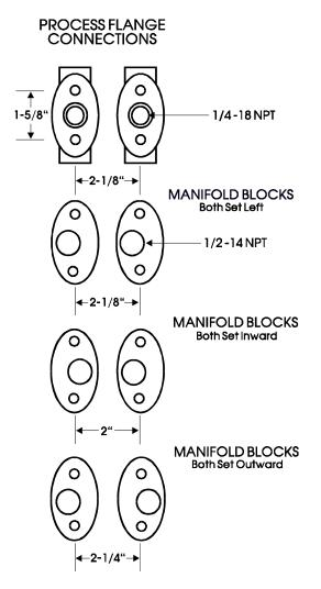
Figure 1A-5 - Process Flange and Optional Manifold Block Connectors
