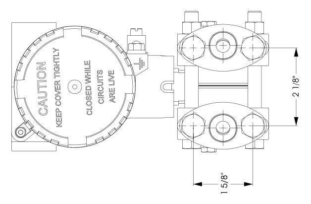
Figure 1A-4C - Dimensions for Series PX771A Transmitter (With Manifold Adapter Option)
