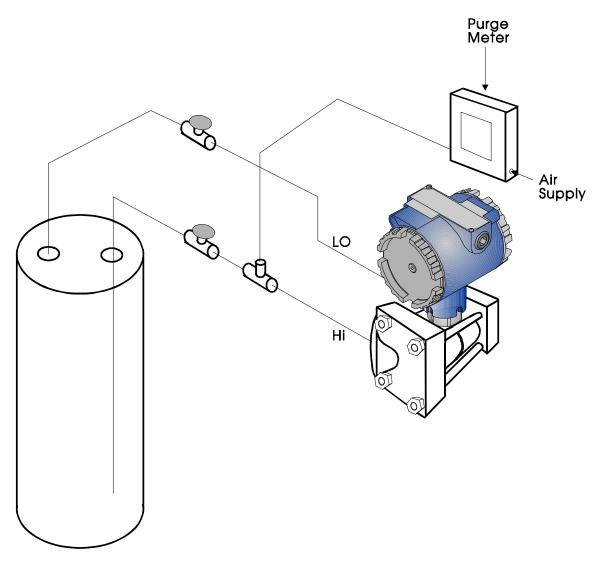
Figure 1A-15 - Closed Tank with Air Purge
