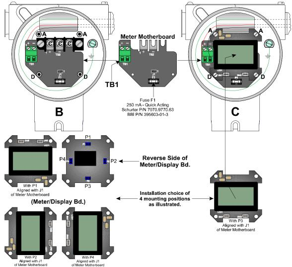
Figure 2-2 - Loop Powered Indicator Installation Diagram
