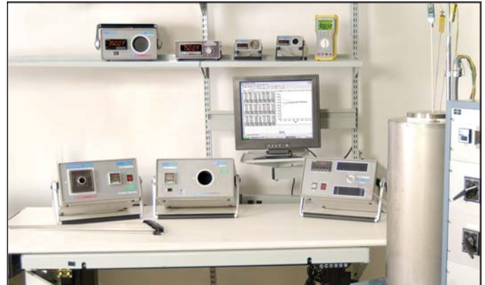
In OMEGA’s calibration laboratory, NIST-traceable precision instruments are used to perform accurate temperature calibrations.
