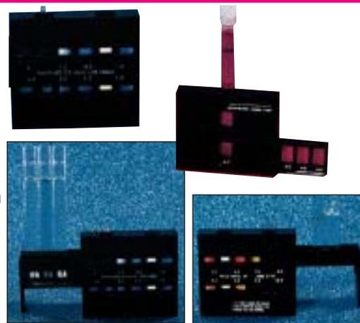
There are two accessories which can be used with an Octet Comparator. The Bi-Color Reader neutralizes sample color and/or turbidity to give more accurate readings. The Axial Reader uses a mirror to extend the view path and intensify the faint colors of low concentrations for easy distinguishing. Both accessories attach directly to the comparator and come with complete instructions for use.
